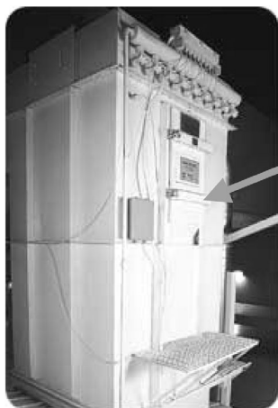
FIGURE 6-7. Side access, bottom bag removal design
