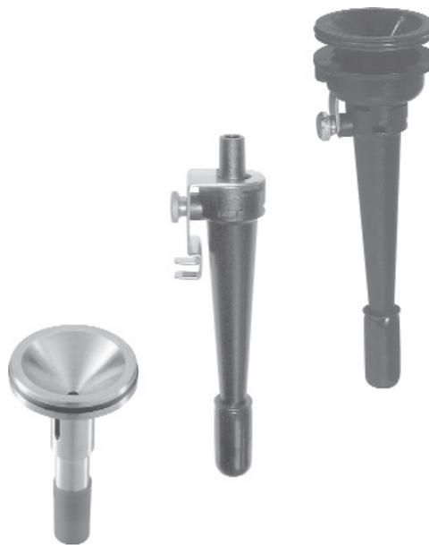
**Figure 24-15.** The SKC aluminum, the 1-hole inlet (simulates the Dorr-Oliver), and the 3-hole inlet cyclones (courtesy SKC, Inc.).
