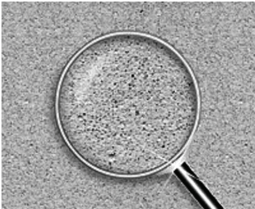
Fig. 1.1—Macroscopic cellular (void) structure of AAC.
