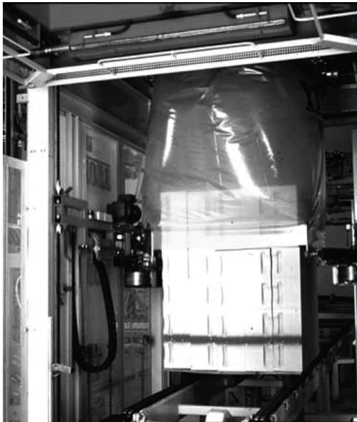
Fig. 3.5—Packaging of finished AAC units.
