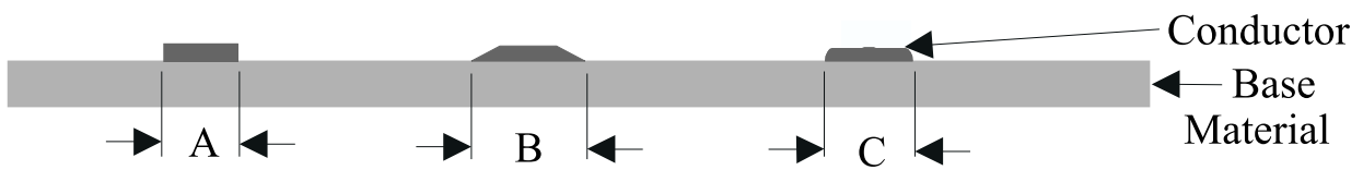
Figure 12.1 Measuring Conductor Trace Average Width (Side-View)
